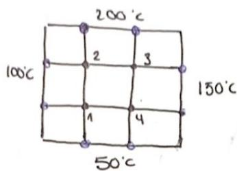
It is a plate with thermal conductivity that is constant, ( $K$ ) and no source of heat.
