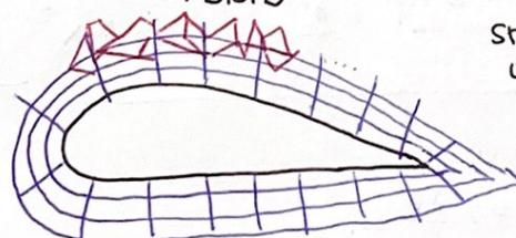
It integrates the structured meshes & the unstructured ones in an efficient manner.
